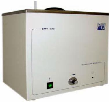
Copper strip corrosion apparatus
